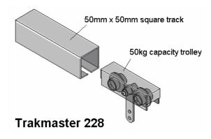
**Trolleys** consist of two sets of wheels and a central swinging pendant. Each trolley has a load capacity of 37kg (152), 50kg (228), or 250kg (406). Twin trolleys may be used connected by a stabilised cross bar allowing a choice of load attachments. Index rotators are
