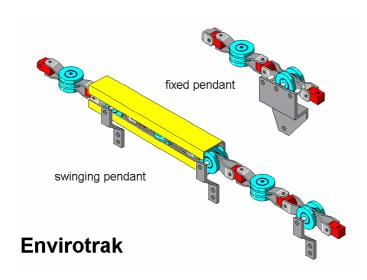
The conveyor is designed for medium duty loads (approx. 25kg per pendant) and is is quiet running.
