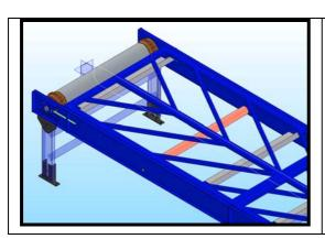
Flat belt conveyors can be made in a variety of lengths widths and work heights. The conveyor is built onto a mild steel welded free standing structure. The conveyor has a mild steel headshaft, keywayed where necessary to fit toothed cast iron sprockets, as well as a split tailshaft. All shafts are supported in sealed for life self aligning ball bearings and include tensioning arrangements.
