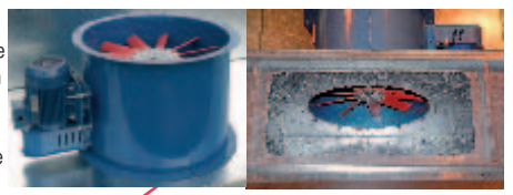
Most fan cases have integral access doors.
